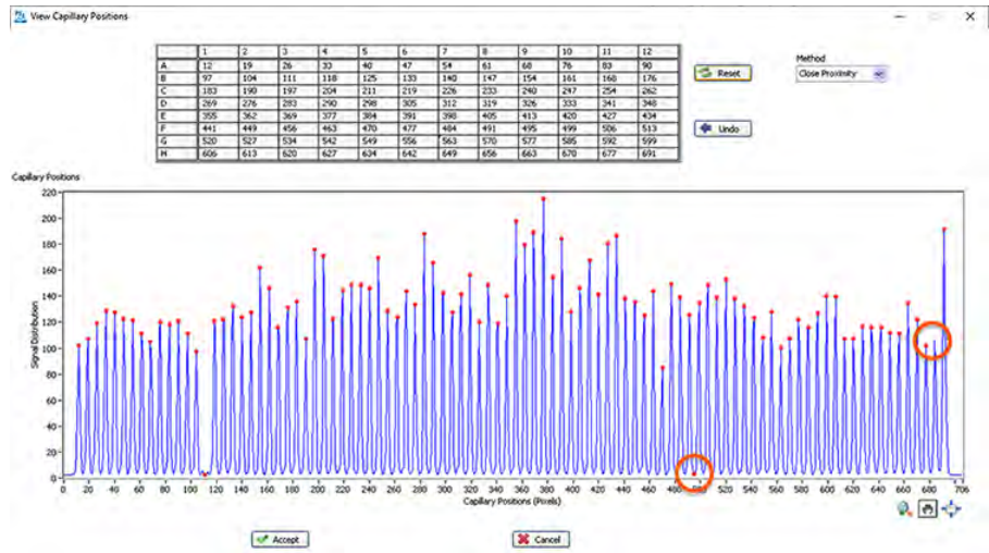
Figure 95 View Capillary Positions window where capillary is not assigned properly (circled in red)
