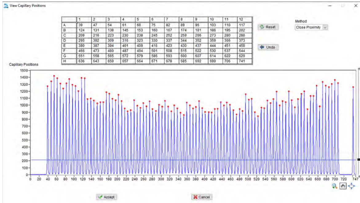
Figure 94 Capillary Positions window after pressing Reset . A blue horizontal cursor can be used to select the threshold for locating capillary positions.
