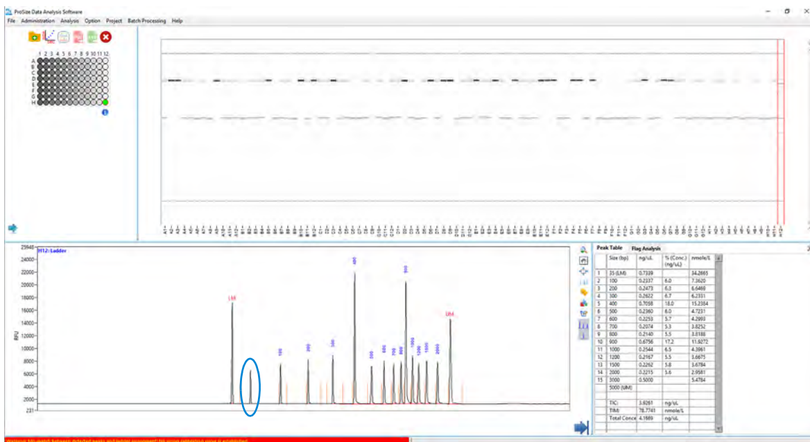
Figure 61 Main screen showing improperly fitted size calibration (not enough integrated peaks). Solution to correct: In the Peak Analysis table lower the Min. Peak Height (RFU) threshold to integrate missing peak (circled in blue).
